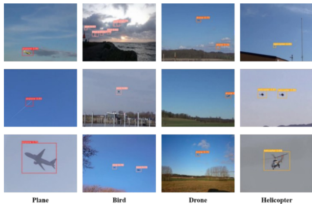
Fig. 11 Illustration of detection results on a multiclass RGB dataset
